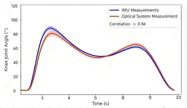
Note. This figure depicts the knee joint angle over time in the sagittal plane, comparing measurements from Inertial Measurement Units (IMUs) and a gold-standard optical system. The correlation coefficient between the two measurement methods exceeds .94, demonstrating the high accuracy of IMUs in capturing knee joint kinematics, consistent with the findings of (Di Paolo et al., 2021).
