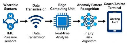
Note. This schematic illustrates the sequential process of the AI-enabled injury warning system, encompassing wearable sensor data acquisition, edge computing-based real-time analysis, anomaly pattern recognition via injury risk algorithms, and feedback delivery to coach/athlete terminals.
