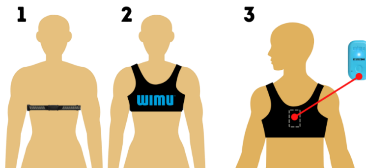
Figure 2. Placement of the heart rate monitor and the inertial device (own elaboration). 1 and 2: Front view; 3: Rear view.
